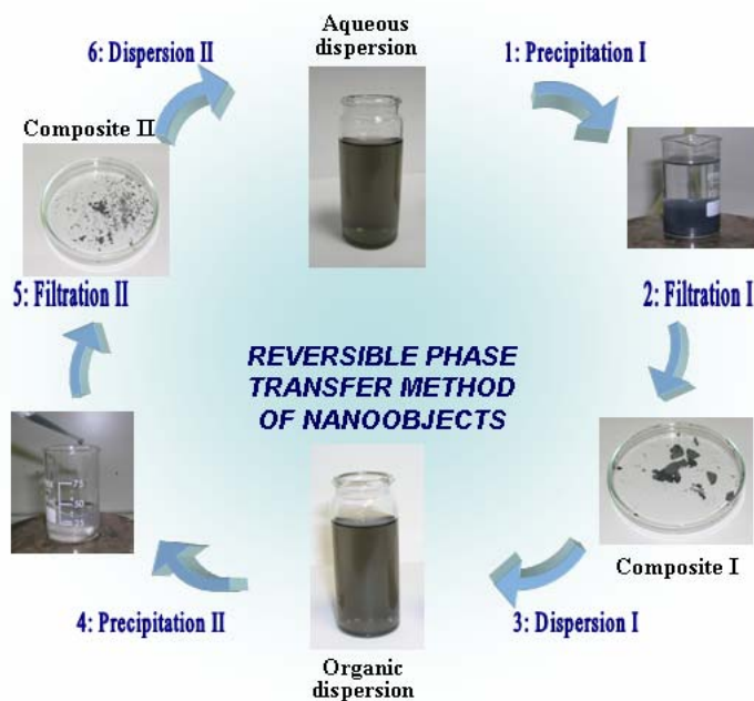
Figure 2. Method for the reversible transfer method of nano-objects between aqueous and organic phases using polymeric ionic liquids
