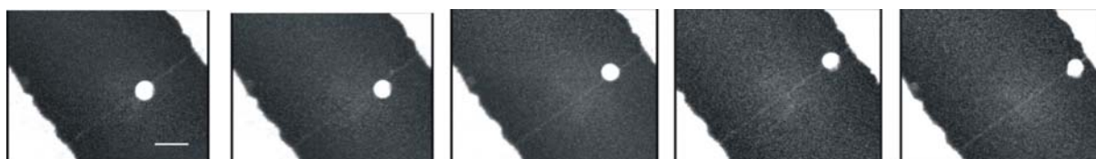
Fig. 2. Translational motion. Top down SEM images where the gold cargo is moving along the nanotube. The motion is actuated by passing a large electrical current through the nanotubes. Note that the driving mechanism for the motion is not due to electromigration, but comes from the thermal gradient along the nanotubes (induced by the electrical current). The metal plate, which initially had a rectangular shape, melted through Joule heating, and became a ball. The scale bar is 400 nm.
