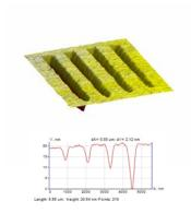
Figure 4 Ultra Shallow scratches in order of nm to find the scratch hardness of the low k materials
