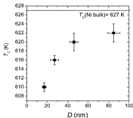
Fig. 4. Curie temperature evolution for samples with different nanowire diameters.
