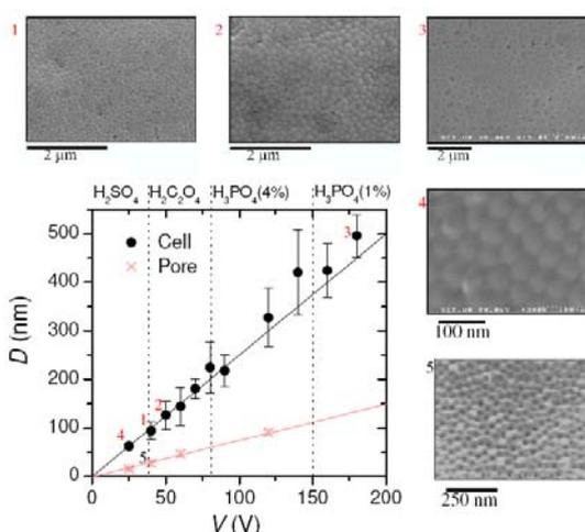
Fig. 2.. Voltage influence on cell and pore diameter. Temperatures and electrolytes used are described in table 2.2 and marked in superior scale. For all samples:  $t_1=30$  min and  $t_2=120$  min. Black and red lines are linear fits for cell and pore diameters respectively.
