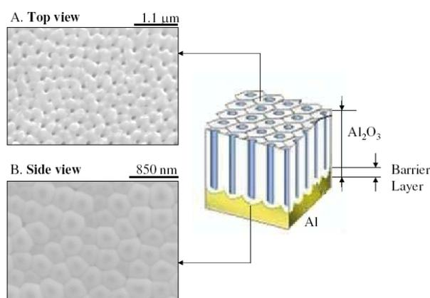
Fig. 1. Schematic drawing of the nanoporous alumina structure as obtained as a result of anodic oxidation. Example of the top view (A) and the side view after aluminium removal (B) of a sample synthesized at 160 V during 2 hours in H<sub>3</sub>PO<sub>4</sub> 1%.
