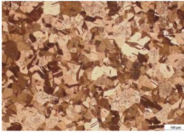
**Fig. 2** Microstructure of pure copper after annealing at 600°C for 2 hours.
