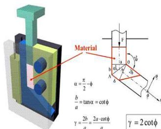
**Fig. 1** Test system of the equal-channel angular pressing.
