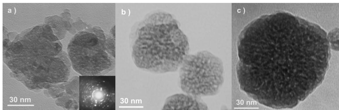
Figure 1. TEM images of nanoporous BaTiO<sub>3</sub> prepared with PE 10300: a) as-synthesized crystallites (selected area electron diffraction is shown as inset); b) calcined at 573 K and c) calcined at 673 K.
