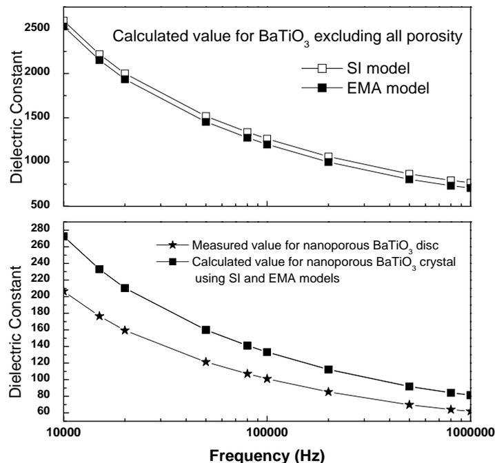
Figure 2. Dielectric characterization on isostatic pressed discs composed of nanoporous BaTiO<sub>3</sub>, based on which, the apparent dielectric constants of nanoporous BaTiO<sub>3</sub> crystallites and BaTiO<sub>3</sub> without any porosity are estimated using both SI and EMA models. For nanoporous BaTiO<sub>3</sub> crystallites, using SI and EMA results in very close values.
