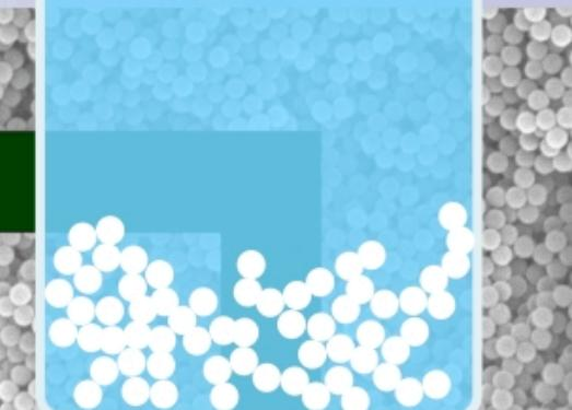
The colloid is in a subtle equilibrium between Coulomb (repulsive) and van der Waals (attractive) forces. Addition of salt to the colloid collapses the double layer and disrupts the rheological equilibrium. That is, particles coagulate and sediment in a rapid and disorderly manner.
