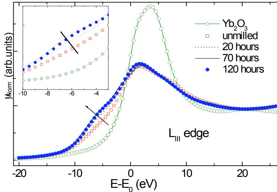
The XANES signal reveals clearly a change in the electronic configuration, with a modification of the valence
