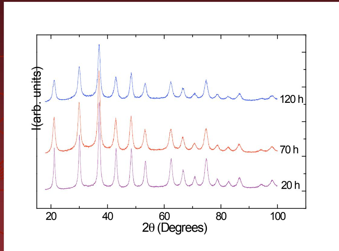
**Rietveld analysis:** Cubic structure  $a = 4.2057(7) \text{ \AA}$ , constant lattice parameter, line broadening due to size decrease and strain effects
