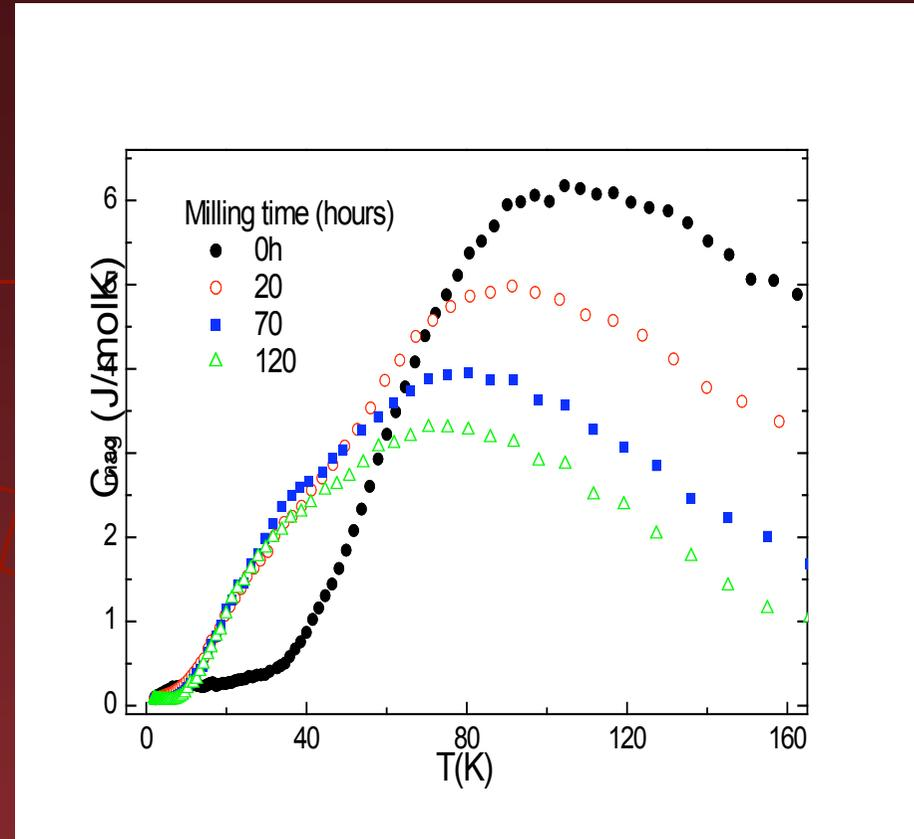
**We have produced non-magnetic isostructural  $\text{LuAl}_3$  to obtain the magnetic  $C_p$**
