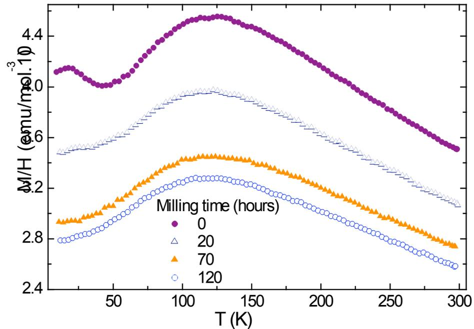
**With the increase of milling time the magnetic signal (susceptibility =  $M/H$ ) becomes weaker towards the non-magnetic state**
