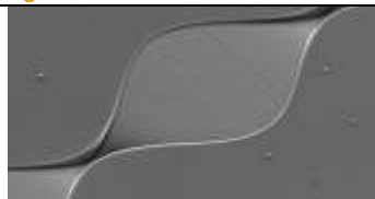
Figure 1: True 3D in one go: micro-fluidic mixer by simultaneously controlling both lateral shape and depth of the structure, fabricated with FIB.
