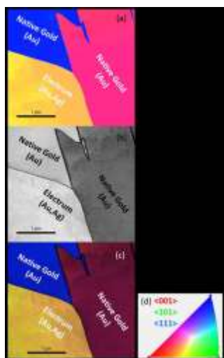
Figure 1: Gold crystal orientation maps obtained by means of PED (a) zone axis identification distribution yellow (4 1 9) blue (8 7 9) and pink (-3 -2 -9), (b) the goodness of fit map in grayscale showing the darkest areas that correspond to the grain boundaries with unassigned zone axis, (c) composite image with zone axis identification and goodness of fit and (d) zone axis and the corresponding color scale.
