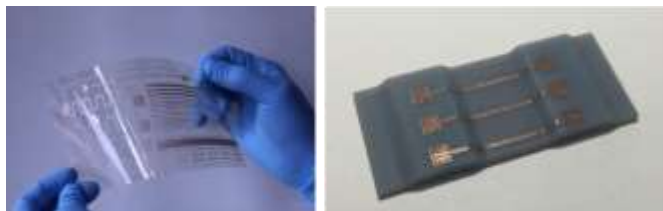
Figure 1: Ink-Jet printed copper pattern on PET film (left), and on 3D printed plastic object (right)
