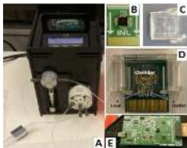
Figure 1: Detection module, A) Flow injection system; B) multi GFET chip; C) PDMS chamber; D) PDMS/GFET chip; E) platform readout.
